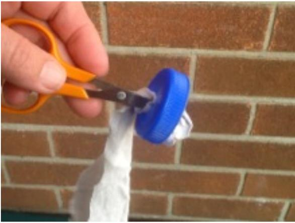
4. Remove the lid of the bottle and place it top-side up on the work surface. Now use the bradawl or other cutting tool to make a hole in the lid big enough to get your wick through. Use the same tool to push a corner of the wick through the gap and then pull it through, rather than making a really large hole. You need to pull through enough wick to nearly reach the level of the cut edge of the bottle. Replace the lid on the bottle top.
